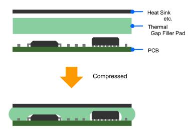
GR-Sd is the lowest modulus type of Gap Filler Type available. Ideally suited for applications requiring low compression force on the component. It offers the high performance that very easily conforms in and around protrusions and depressions on components to make complete, reliable physical contact.
